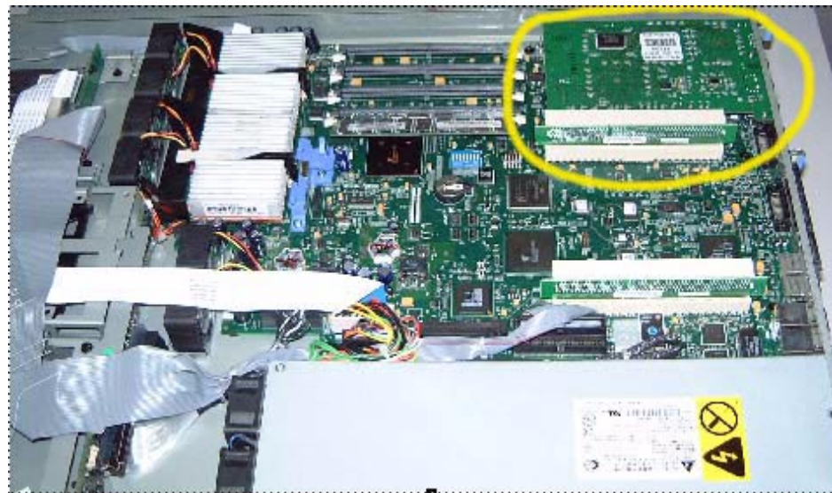
Figure 5-3 x330 with Myrinet card installed into short PCI slot
